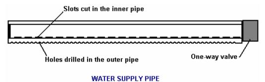
This water supply pipe arrangement works well in practice and it looks surprisingly like the gas take-off pipe which has a series of holes drilled along the top of it:
