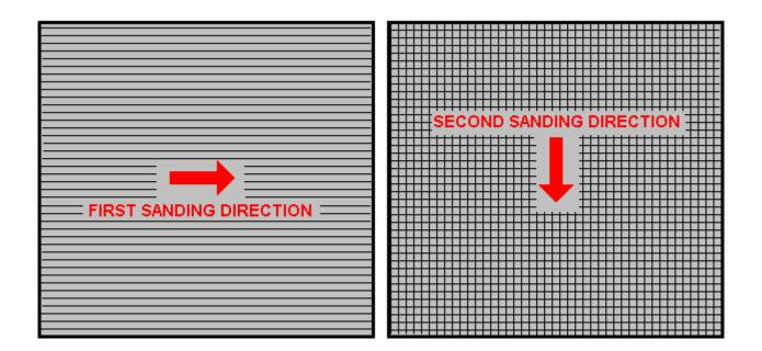
Bob uses a 6-inch x 48-inch belt sander which is great for preparing the plates and he uses it all the time now with 60 or 80 grit. Always wear rubber gloves when handling the plates to avoid getting finger marks on the plates. Wearing these gloves is very important as the plates must be kept as clean and as grease-free as possible, ready for the next stages of their preparation.
